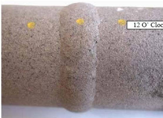
Figure 6a: Sand Blasted Surface of 347H after 8,596 service hours
