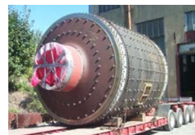
Replacement Ball Mill Drums
