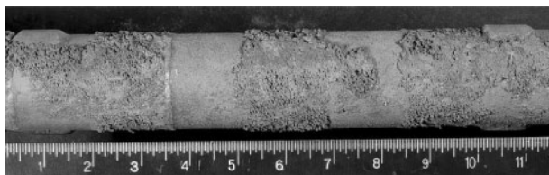
3 One year corrosion probe from zone 2, mid-western utility: post-exposure (before cleaning)
